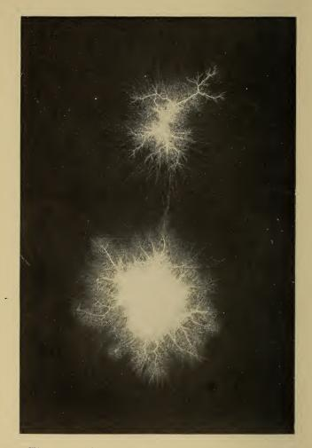
The above is a reproduction of a photograph of an electric spark, showing the Negative and Positive. The white represents the negative, the lines show the positive, the view on the top showing the strongest positive effect.
