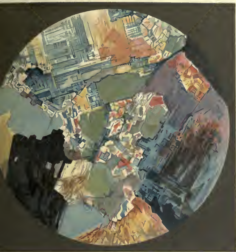
Thin section, in polarized light, of a portion of the Shaft of the Egyptian Obelisk erected in Central Park, New York.
